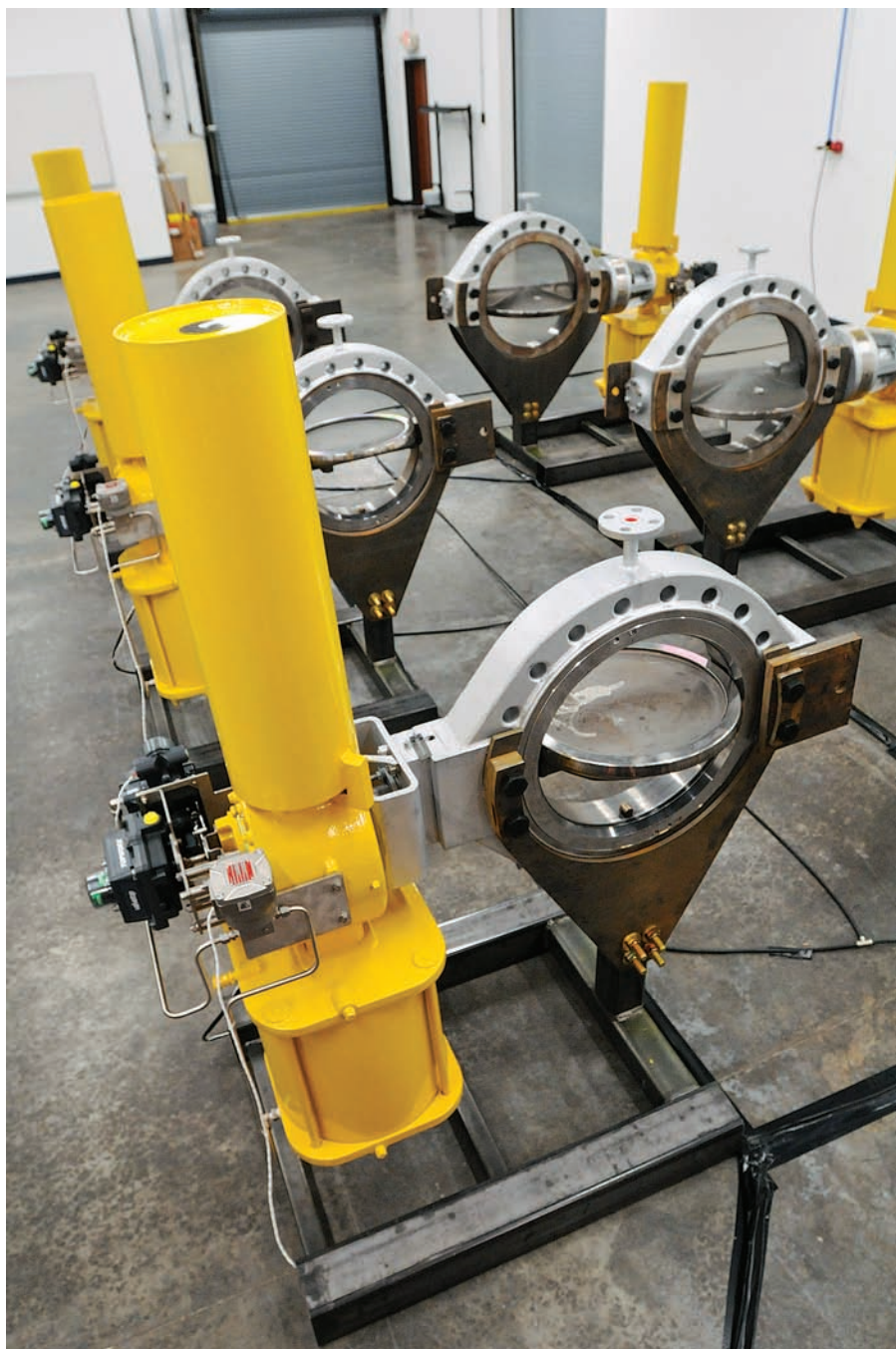
FIG. 2. Tail gas diverter valves prior to installation.
